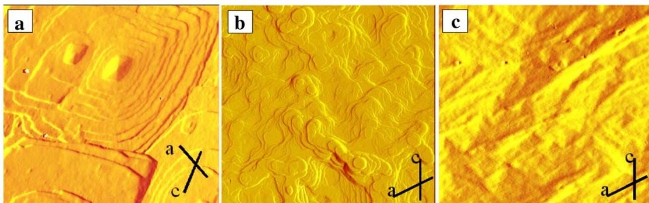
**Fig. 5.** AFM images of the acetaminophen (010) face etched by **a** 25 mg/ml PVA(15 K), **b** 12.5 mg/ml PEG(1000) and **c** 1 mg/ml PVP(K30). The *a* and *c* axes were marked on corresponding images. All scan sizes were  $20 \times 20 \mu\text{m}$ .
