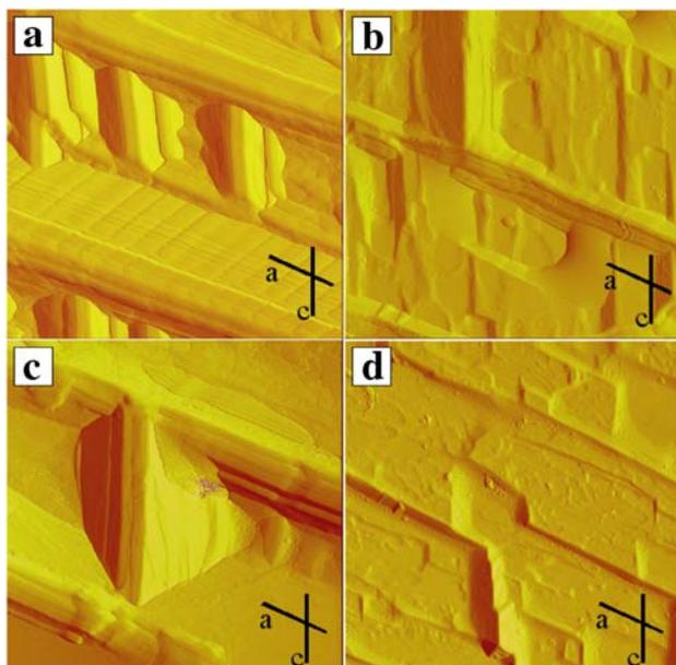
**Fig. 3.** AFM images of the acetaminophen (010) face etched by **a** water as well as 100 mg/ml **b** glucose, **c** sucrose and **d** 2-pyrrolidinone aqueous solutions. The *a* and *c* axes were marked on corresponding images. All scan sizes were  $5 \times 5 \mu\text{m}$ .
