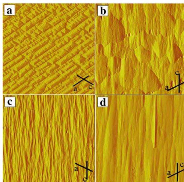
**Fig. 4.** AFM images of the acetaminophen (010) face etched by **a** 10 mg/ml Dextran (52.9 K), **b** 10 mg/ml HEC(90 K), **c** 10 mg/ml HPC(80 K) and **d** 1 mg/ml HPMC(E4M) aqueous solutions. The *a* and *c* axes were marked on corresponding images. All scan sizes were  $20 \times 20 \mu\text{m}$ .
