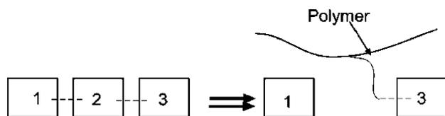
Fig. 1. Polymer forms a hydrogen bond with acetaminophen on crystal surface. The dotted lines represent hydrogen bonds.
